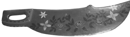
Scutching knives were used to separate the woody stalk of the flax from the interior fibers to prepare the flax for spinning.
